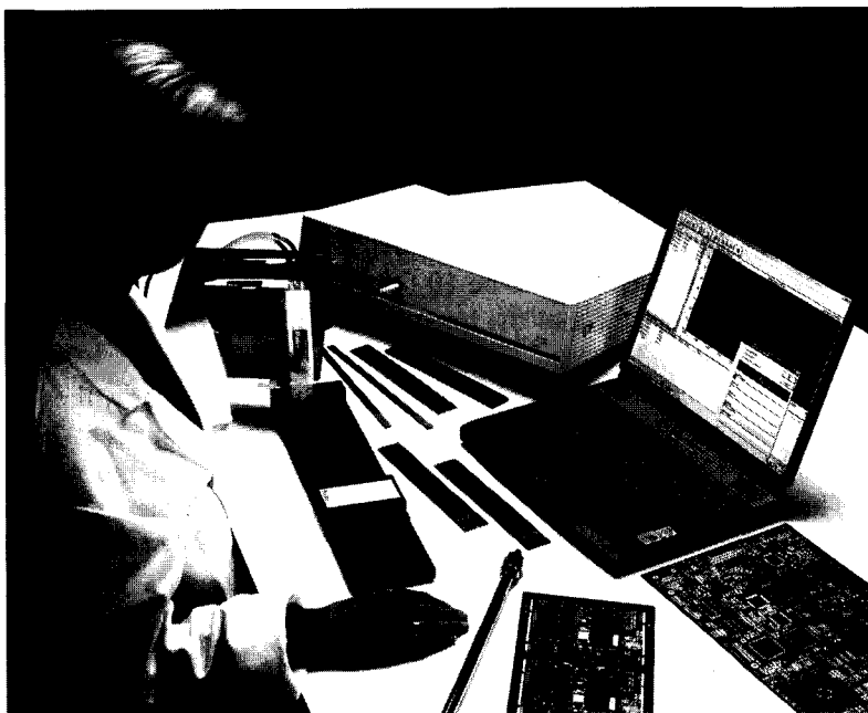
Figure I-2 Polar Instruments CITS500s TDR measuring system using a standard PC for data analysis, processing, and display (courtesy Polar Instruments).
