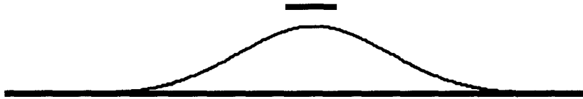
Figure 16-1 Current distribution of a return signal spreads out on the plane underneath the signal trace.
